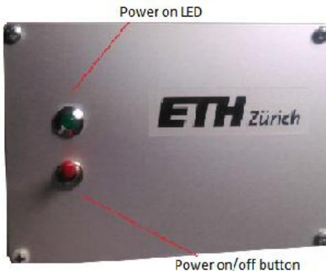
Figure 3(a). Front panel of the CALLISTO
